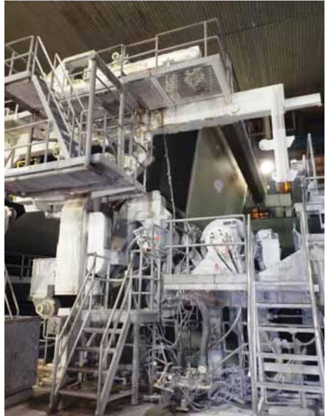
Most of the existing press section arrangement was eliminated, and the new section is currently a single-felted, single pressure roll configuration.
