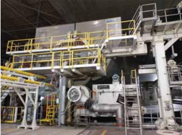
The 12-ft.-dia. PMT yankee dryer, a grooved cast iron unit with six condensate headers, was shipped from Europe, unloaded at Norfolk, Va., and delivered by truck to the mill.
