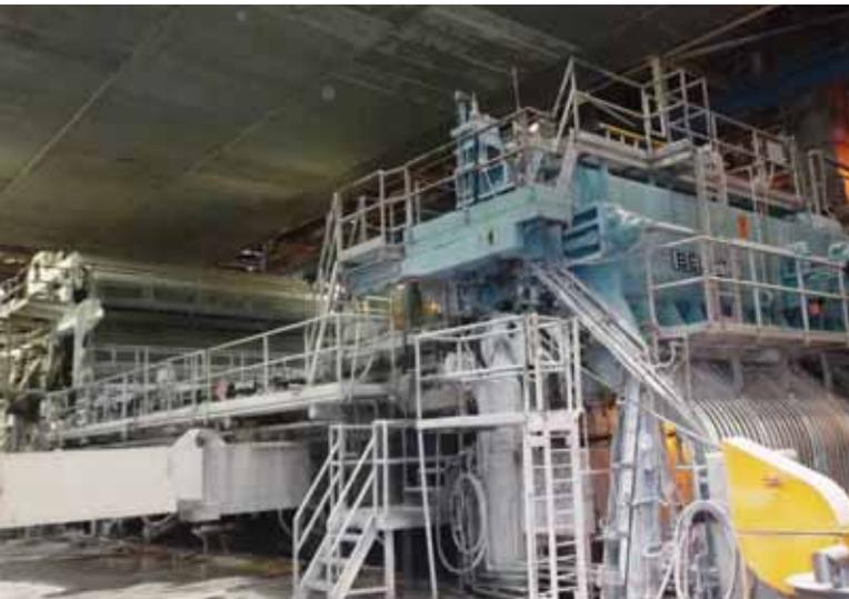
In the conversion, the forming section was basically retained, with only minor modifications to the forming board and decommissioning of about half the vacuum.
