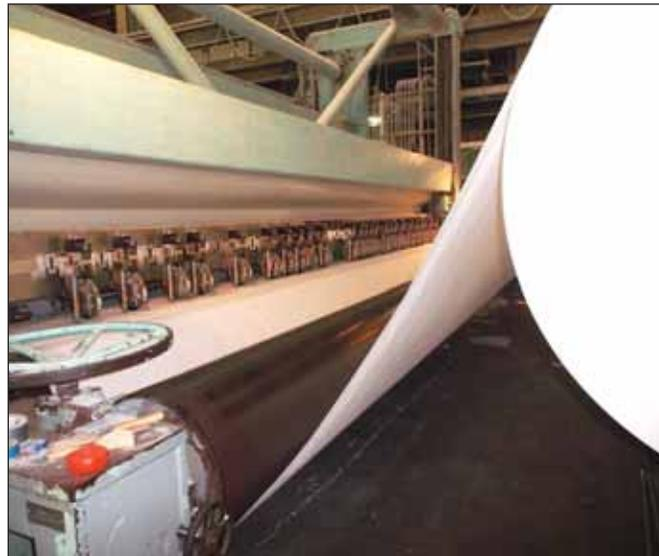
The slitter rewinder can produce various sized rolls at diameters up to 68-in., with width dependent basically on the size of the truck.
