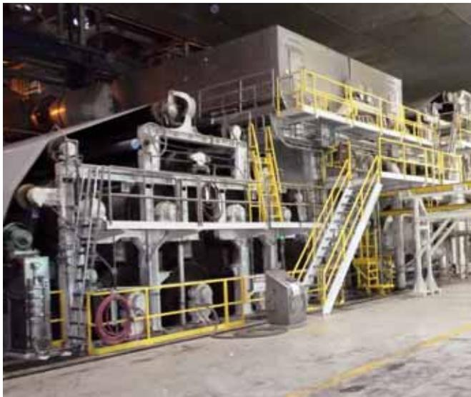
The after-dryer section is comprised of eight dryer drums from the existing fine paper dryer section that were reconfigured and set up to handle tissue.
