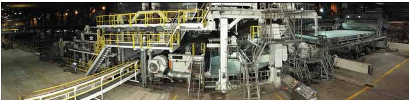
Wide-angle view of PM 6, with the fourdrinier forming section on the right, yankee dryer and hood in the center, and after-dryer section on the left.
